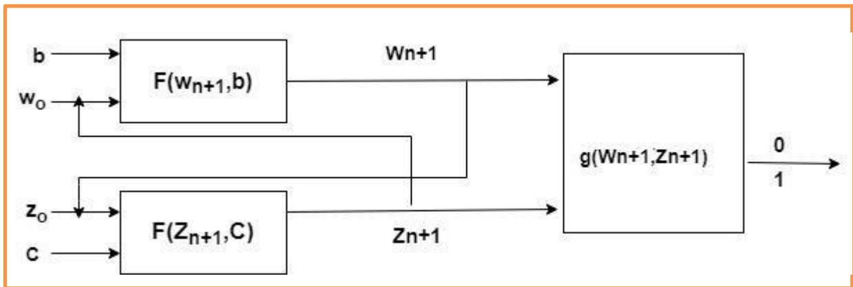
Figure (3.3) The Block Diagram of Random (K)
